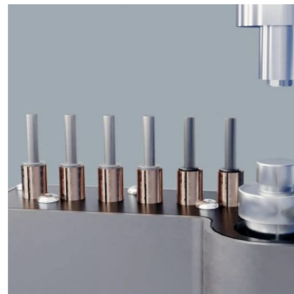
6 tools 4 zirconia mill+2 resin mill
